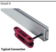
Most horizontal extrusion connections have a patented expandable lock. This lock inserts into the groove of an opposing extrusion. Tightening the lock with the Hex Key Tool expands the lock and creates a strong positive connection.
