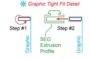
Note: When applying SEG graphic along the bottom of curved extrusion #5, double over the silicone edge of graphic for tight fit.
