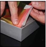
Step 1 Insert corner A. Turn edge of of welt with fabric to outside the corners. into the channel. Repeat for other side of this corner.
